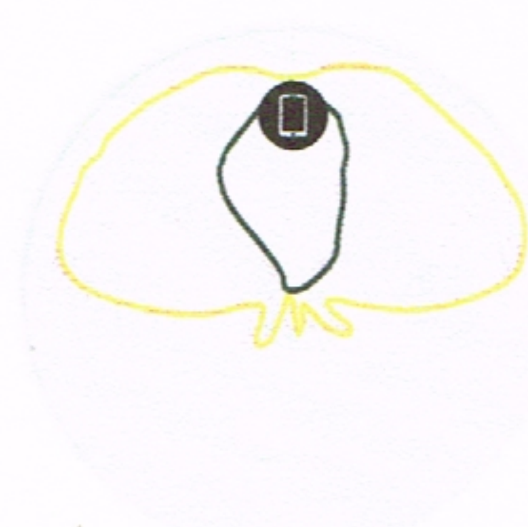
Figure 4 - T310d 2.4GHz Elevation Antenna Patterns
